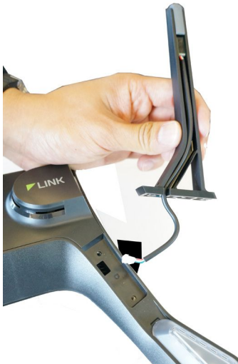
Figure 10.4.3.2: Insert New Leg with Compass
