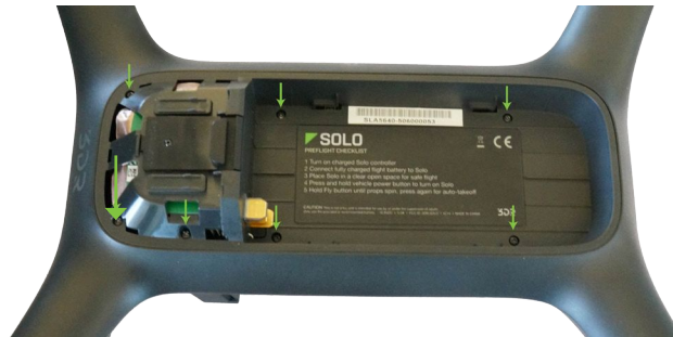
Figure 10.5.2.1: Battery Tray Removal
