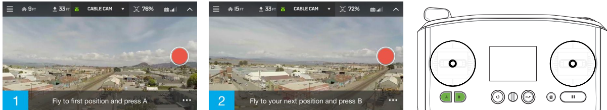
Figure 6.2.1.1: App - Cable Cam Setup
