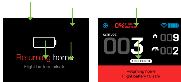
Figure 7.2.5.2: Controller - Critical Battery Alert
