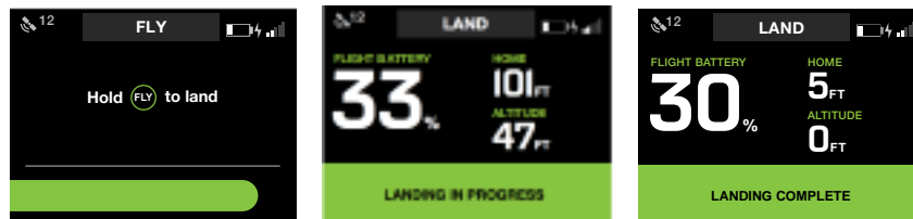
Figure 5.3.1: Controller - User-Initiated Landing
