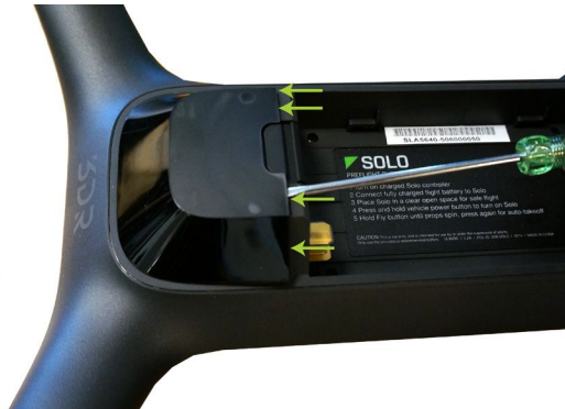
Figure 10.5.1.1: GPS Cover Removal
