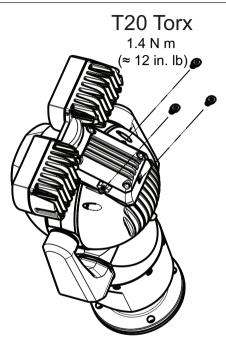
6. Partially engage the threads of all three (3) screws. Do not tighten any one screw completely at this point.
