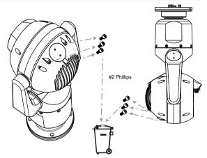
2. Remove and discard the three (3) plastic screws surrounding the appropriate access port where the illuminator will be installed.
