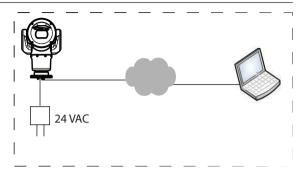
From the web browser, access the camera's Settings page. Select Advanced > Camera > Installer Menu > Orientation, and then select "Inverted". Click **Set** to confirm the selection. The camera head will rotate automatically into inverted position (180°). Regardless of mounting orientation, the visor should always be above the camera window.
