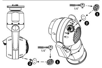
3. Remove the appropriate access plug from the camera head, using a ¼ in. drive wrench (not supplied) with the spanner tool (supplied). For upright cameras, remove the plug near the visor. For inverted cameras, remove the plug farther away from the visor.
