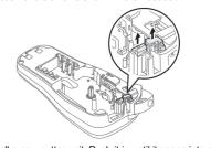
2. Install a new cutter unit. Push it in until it snaps into place. ♠ Do not touch the cutter blade directly with your fingers.
