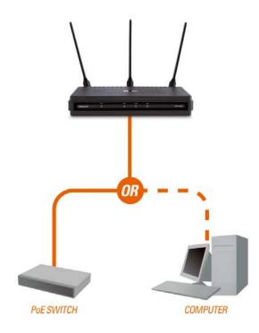
Connect one end of an Ethernet cable (included with your package) to the LAN port on the DAP-2553 and the other end of the Ethernet cable to either your computer or to your PoE switch. The AP can be powered on by a PoE switch or by the power adapter shipped with the AP.
