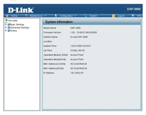
Alternatively, click the "Save and Activate" option on the Configuration drop-down menu at the top of each DAP-2690 window. This will cause the DAP-2690 to save and reboot.
