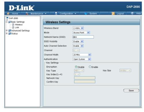
Channel Width: Allows selection of the channel width you would like to operate in. 20 MHz and Auto 20/40 MHz allow both 802.11n and non-802.11n wireless devices on your network when the wireless mode is Mixed 802.11 b/g/n in 2.4G and Mixed 802.11 a/n in 5G. When the channel width is set to Auto 20/40 MHz, then 802.11n wireless devices are allowed to transmit data using 40 MHz.
