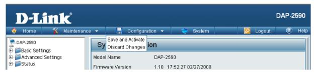
The drop-down Configuration menu allows users to save the current changes and reboot the DAP-2690 by clicking "Save and Activate".
