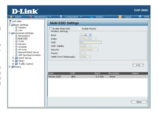
Priority: When the Enable Priority check box is checked at the top of this window, this drop-down menu is used to select a priority between **0** and **7**.
