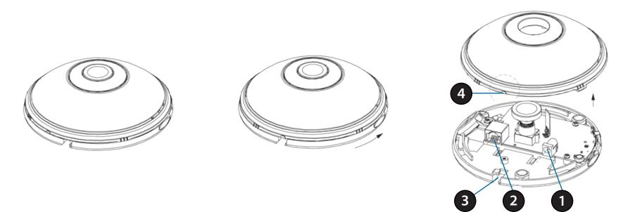
You can access the inside of the DCS-6010L by rotating the camera cover counter-clockwise, then lifting it off of the camera.
