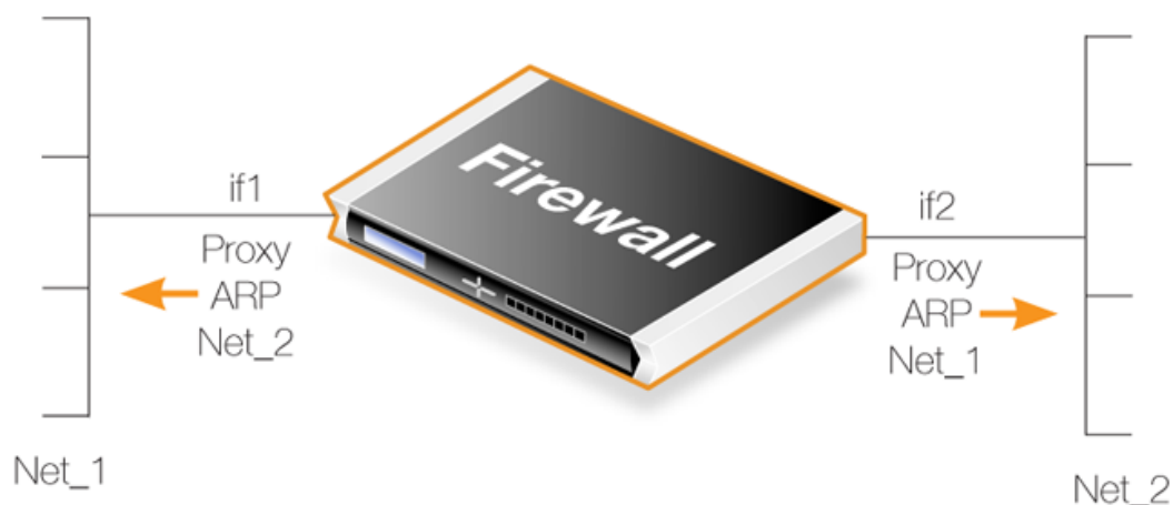
Figure 4.4. A Proxy ARP Example
