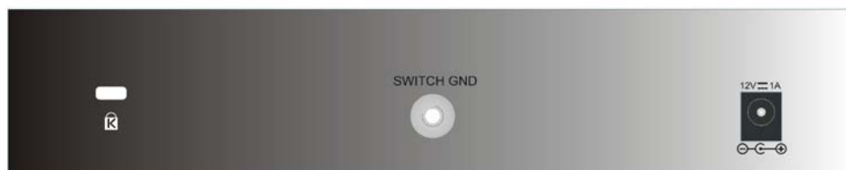
Figure 1.2 – DGS-1100-06/ME Rear Panel
