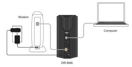
6 After the router has powered up, verify that the Power (green) and Internet (orange or green) LEDs are both lit then continue with the Configuration section on the other side.
