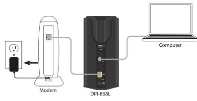
**5** Plug the power adapter into your router and connect to an available power outlet or surge protector. If the Power LED does not light up, press the Power button on the back of the router.
