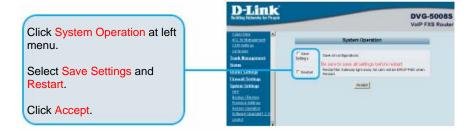
Once the unit reboots you will see the message. Check to see if the status LED light goes from blinking green to solid green on the front panel of the DVG-5008S.
