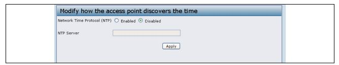
Figure 24: Enabling Network Time Protocol Server
