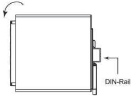
To remove the Moxa EDS-600 switch from the DIN-Rail, use a screwdriver to push down the spring-loaded bracket until it locks in place, as shown in the following diagram. Next, rotate the bottom of the switch upwards and then remove the switch from the DIN-Rail.
