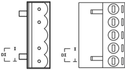
**STEP 1:** Insert the negative (ground)/positive DI wires into the  $\perp$ /I1 terminals, respectively.
