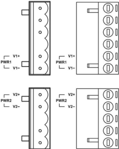
**STEP 1:** Insert the negative/positive DC wires into the V-/V+ terminals, respectively.
