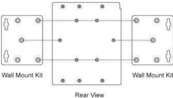
**STEP 2:** Mounting the EDS-600 on the wall requires 4 screws. Use the EDS-600, with wall mount plates attached, as a guide to mark the correct locations of the 4 screws. The heads of the screws should be less than 6.0 mm in diameter, and the shafts should be less than 3.5 mm in diameter, as shown in the figure at the right.
