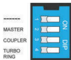
The default setting for each DIP Switch is OFF. The following table explains the effect of setting the DIP Switch to the ON position.
