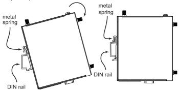
To remove the OnCell G3150A-LTE from the DIN rail, reverse steps 1 and 2 above.
