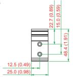
The OnCell G3150A-LTE Series computers come with a DIN-rail kit attached to the back panel. Mount the OnCell G3150A-LTE Series on corrosion-free mounting rails that meet the EN 60715 standard.
