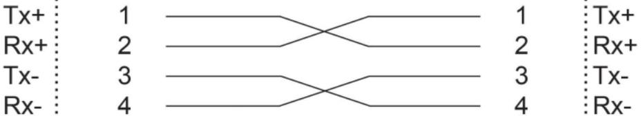
**M12 (4-pin, M) to M12 (4-pin, M) Straight-Through Cable Wiring**
