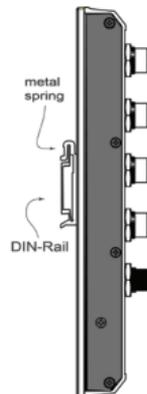
To remove the Moxa ToughNet Switch from the DIN-Rail, simply reverse Steps 2 and 3 above.
