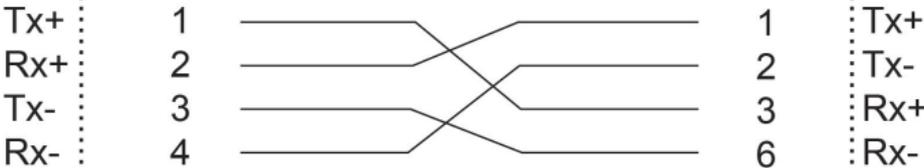
**M12 (4-pin, M) to RJ45 (8-pin) Straight-Through Cable Wiring**
