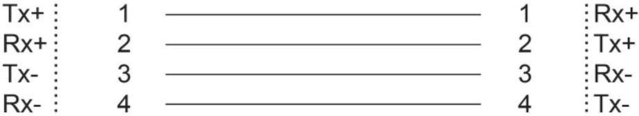
**M12 (4-pin, M) to RJ45 (8-pin) Cross-Over Cable Wiring**
