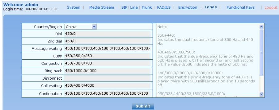
Figure 2-19 Call progress tone configuration interface
