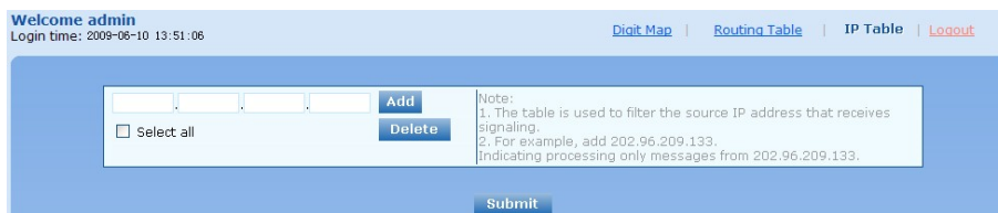
Figure 2-8 Configuration Interface for IP Table
