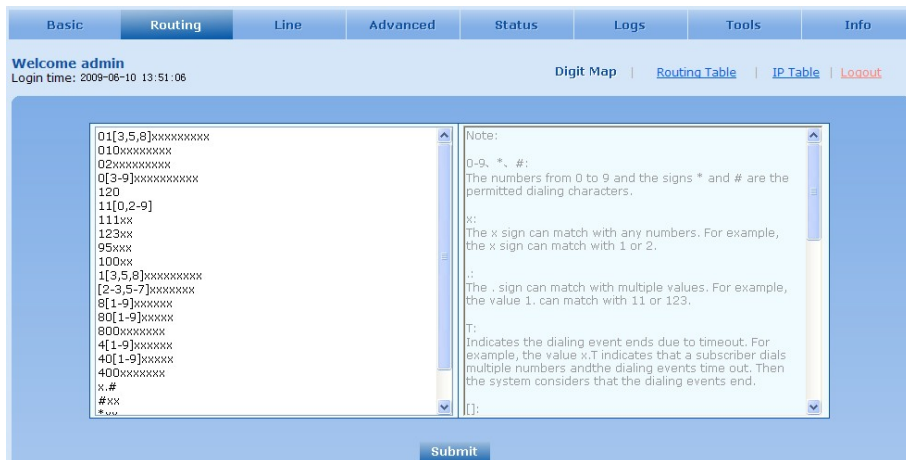
Figure 2-6 Configuration Interface for Digit Map
