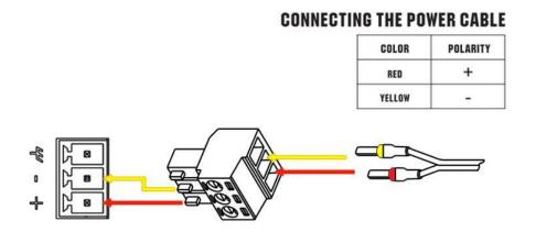
R2000 router supports reverse polarity protection, but always refers to the figure above to connect the power adapter correctly. There are two cables associated with the power adapter. Following to the color of the head, connect the cable marked red to the positive pole through a terminal block, and connect the yellow one to the negative in the same way.
