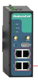
Each Ethernet port has two LED indicators (please check the following picture). The yellow one is **Speed indicator** and the green one is **Link indicator**. There are three status of each indicator. For details please refer to the form below.
