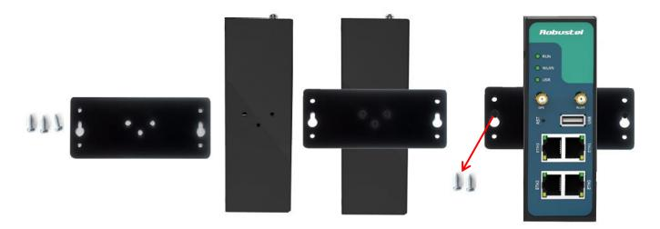
2. Mount the router on a DIN rail with 3 pcs of M3 screws, and then hang the DIN-Rail on the holder. You need to choose a standard holder.
