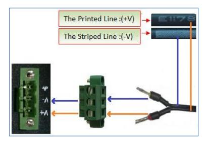
The power supply range is 9 to 60 VDC.
