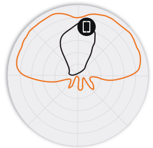
Figure 5 - T310d 5GHz Elevation Antenna Patterns
