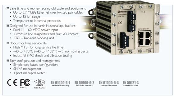
The Wolverine DDW-220 allows effective Ethernet networks to be created over long distances (up to 15 km) at data rates up to 5.7 Mbit/s. The SHDSL technology makes it possible to reuse many types of pre-existing copper cables which can lead to considerable financial savings. Dependent on cable characteristics, distances up to 15 km (9.3 mi) can be achieved. The protocol transparent link allows any industrial protocol to pass unhindered ensuring the unit is easy to use.
