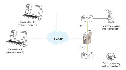
It is also possible to direct the two serial servers to the same serial channel, useful for redundant SCADA.
