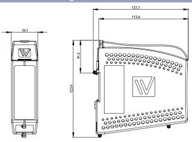
**Dimension W x H x D**  $35 \times 121 \times 119 \text{ mm } (1.37 \times 4.76 \times 4.68 \text{ in})$
