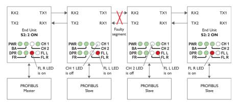
If an optical fibre segment fails, all communication with units beyond the faulty fibre segment will be lost. To determine witch fibre segment has failed, look at the FL L, CH 1 and CH 2 LED's as show in the picture above.
