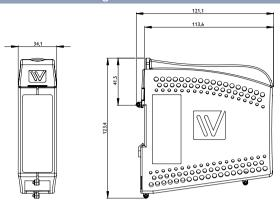
$\textbf{Dimension W x H x D} \qquad \qquad 35 \times 121 \times 119 \text{ mm } (1.37 \times 4.76 \times 4.68 \text{ in})$
