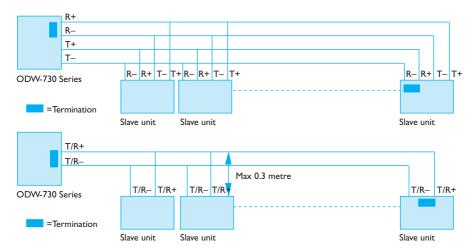
**N.B.** R+/R-,T+/T- definitions are not standard, it can help to shift + and - if the unit does not work.
