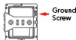
Figure 11 – Connect good earth ground to the AP here
