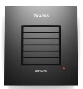
The Yealink DECT repeater can be deployed when there is a desire to extend the range of the W52P, The repeater can also be utilised wherever there is a need to increase limited coverage or improve reception in remote areas.
