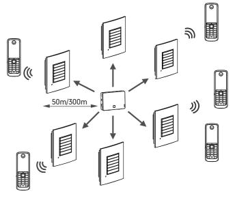
The maximum number of handsets that can be registered to your base station is not affected by the repeater. The repeater can be used to extend the coverage range in all directions, allowing several floors to be covered. The automatic handover process is
