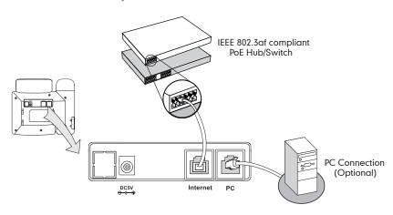
**Note:** If inline power (PoE) is provided, you don't need to connect the power adapter. Make sure the Ethernet cable and hub/switch are PoE compliant.
