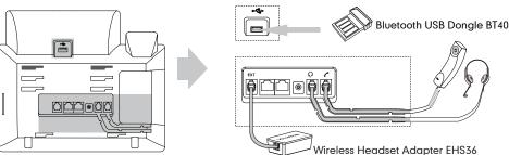
**Note:** The headset, Bluetooth USB dongle BT40 and wireless headset adapter EHS36 should be purchased separately. The EXT port can also be used to connect the expansion module EXP40. For more information on how to use the EHS36, EXP40 and Bluetooth USB Dongle, refer to *Yealink EHS36 User Guide*, *Yealink EXP40 User Guide* and *Yealink Bluetooth USB Dongle BT40 User Guide*.
