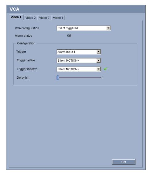
This configuration allows you stipulate that the video content analysis is only to be activated when triggered by an event. As long as no trigger is activated, the **Silent MOTION+** configuration in which metadata is created is active; this metadata facilitates searches of recordings, but does not trigger an alarm.
