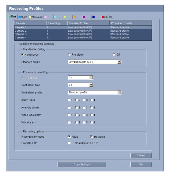
You can define up to ten different recording profiles. You will then use these recording profiles in the recording scheduler, where they are linked with the individual days and times.
