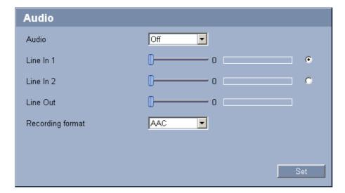
You can set the gain of the audio signals to suit your specific requirements. The current video image is shown in the small window next to the slide controls to help you check the audio source and improve assignments. Your changes are effective immediately.
