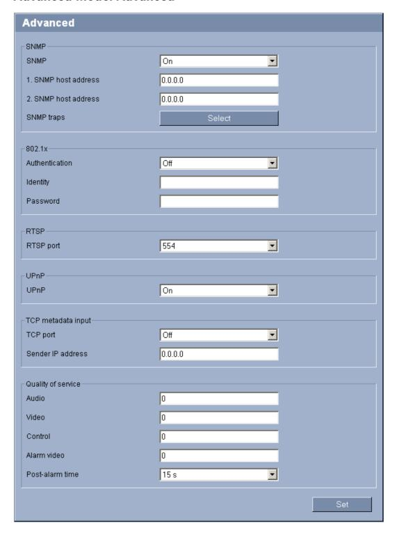
The settings on this page are used to implement advanced settings for the network. Some changes only take effect after the unit is rebooted. In this case, the **Set** button changes to **Set and Reboot**.
