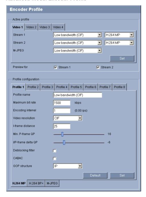
For the video signal encoding, you can select three profiles and a code algorithm for each video input, and you can change the presets for the profiles.
