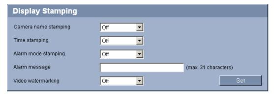
Various overlays or "stamps" in the video image provide important supplementary information. These overlays can be enabled individually and are arranged on the image in a clear manner.
