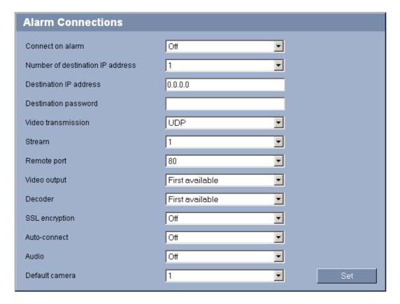
You can select how the VideoJet XF E responds to an alarm. In the event of an alarm, the unit can automatically connect to a pre-defined IP address. You can enter up to ten IP addresses to which the VideoJet XF E will connect in sequence in the event of an alarm, until a connection is made.
