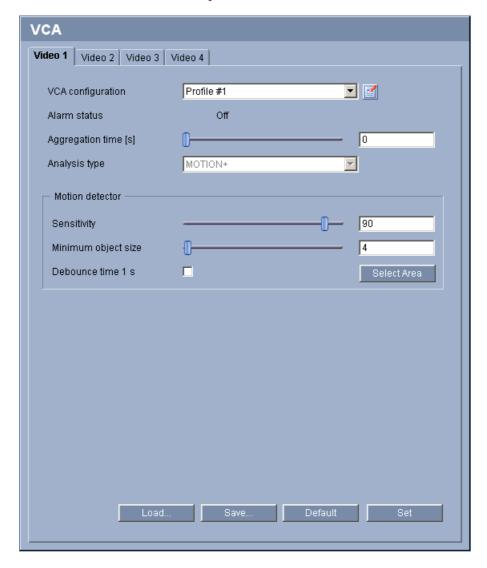
You can configure two profiles with different VCA configurations. You can save profiles on your computer's hard drive and load saved profiles from there. This can be useful if you want to test a number of different configurations. Save a functioning configuration and test new settings. You can use the saved configuration to restore the original settings at any time.
