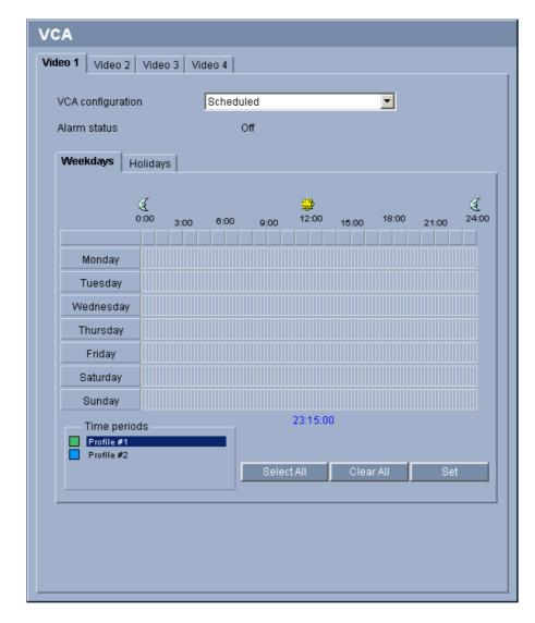
This configuration allows you to link the created VCA profile with the days and times at which the video content analysis is to be active.
