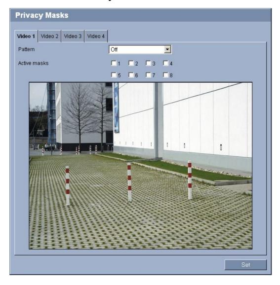
You can cover up to eight different rectangular areas in the video image of each camera, so that private areas are protected in the camera's field of view. This can be useful when public spaces are in the coverage area or monitoring will be limited to a particular zone. The areas covered are indicated by a gray pattern in the video image.
