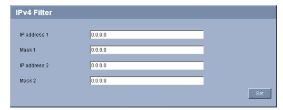
To restrict the range of IP addresses within which you can actively connect to the device, fill-in an IP address and mask. Two ranges can be defined.
