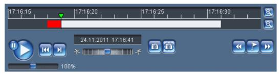
You will see a time bar below the video image for quick orientation. A green arrow above the bar indicates the position of the image currently being played back within the sequence.
