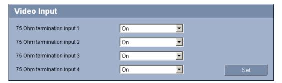
You can activate the 75 Ohm terminating resistance for each video input of the VideoJet XF E. The terminating resistance must be deactivated for the video signal to be looped through. Every video input is closed at the time of delivery.
