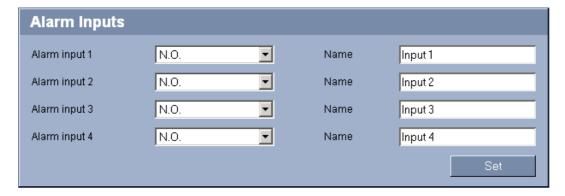
You can configure the alarm inputs of the VideoJet XF E.
