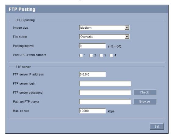
You can save individual JPEG images on an FTP server at specific intervals. You can then retrieve these images at a later date to reconstruct alarm events if required. The resolution corresponds to the highest setting from the two data streams.
