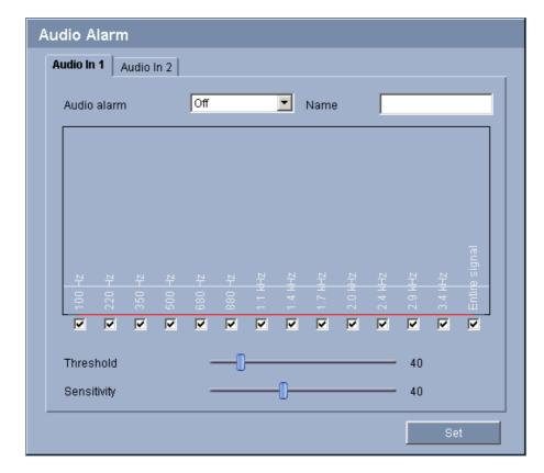
The VideoJet XF E can create alarms on the basis of audio signals. You can configure signal strengths and frequency ranges in such a way that false alarms, for example due to machine noise or background noise, are avoided. Configure the required settings for each audio input. Make sure that you have set up normal audio transmission before you configure the audio alarm here.
