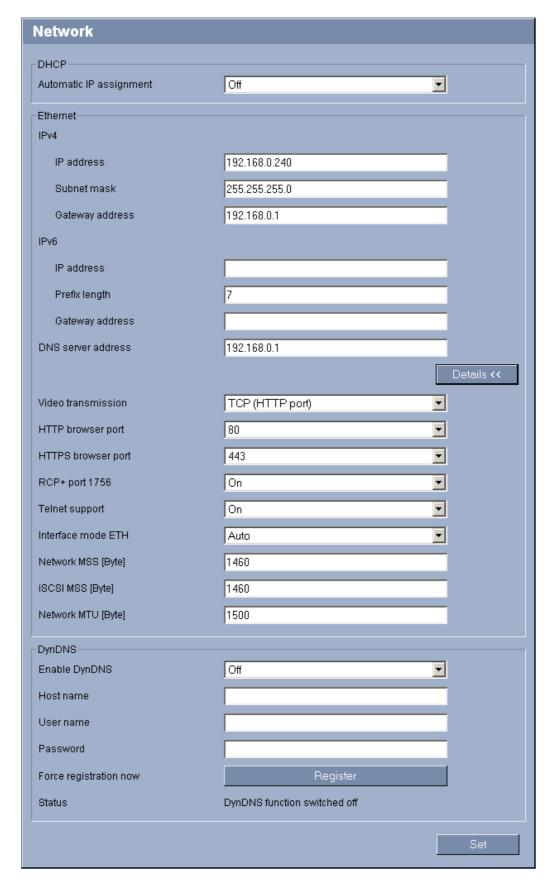
The settings on this page are used to integrate the VideoJet XF E into an existing network. Some changes only take effect after the unit is rebooted. In this case, the **Set** button changes to **Set and Reboot**.
