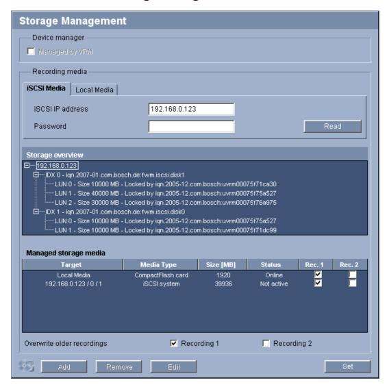
You can record the images from the camera connected to the VideoJet XF E on the local CF card or on an appropriately configured iSCSI system.
