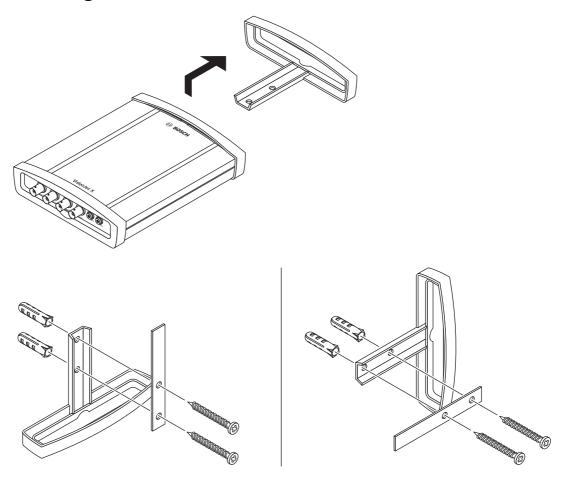
You can secure the VideoJet XF E to walls, below ceilings or any other load-bearing locations using the wall-mounting panel, in either a vertical or a horizontal position.
