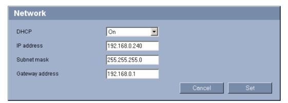
The settings on this page are used to integrate the VideoJet XF E into an existing network. Some changes only take effect after the unit is rebooted. In this case, the **Set** button changes to **Set and Reboot**.
