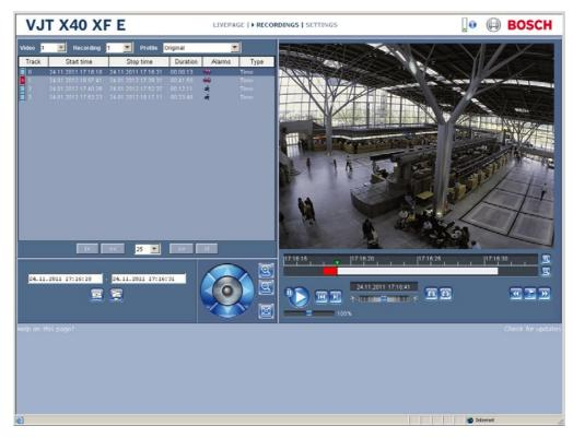
Replay connections utilize the Adaptive Bit Rate encoding capability which automatically adjusts the generated replay data to the available bandwidth. You may also use the built-in transcoding function. Just select any other than the original profile to guarantee smooth replay and browsing through recordings even for bandwidth-limited connections.
