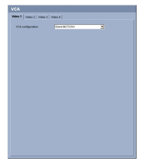
The VideoJet XF E contains an integrated video content analysis (VCA), which can detect and analyze changes in the signal using image processing algorithms. Such changes can be due to movements in the camera's field of view.
