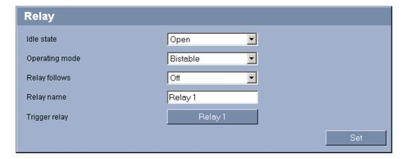
You can configure the switching behavior of the relay output. You can specify an open switch relay (normally closed contact) or a closed switch relay (normally open contact).
