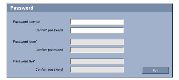
A VideoJet XF E is generally protected by a password to prevent unauthorized access to the unit. You can use different authorization levels to limit access.
