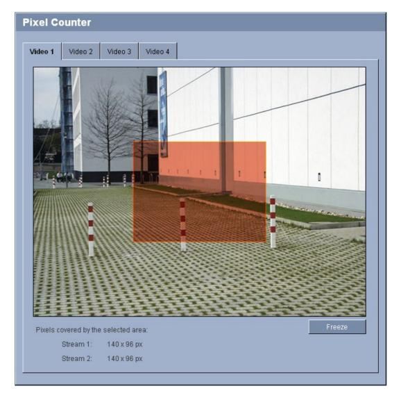
The numbers of horizontal and vertical pixels covered by the highlighted area are displayed below the picture. With these values you can check for each camera whether the requirements for specific functions, e.g. identification tasks, are fulfilled.
