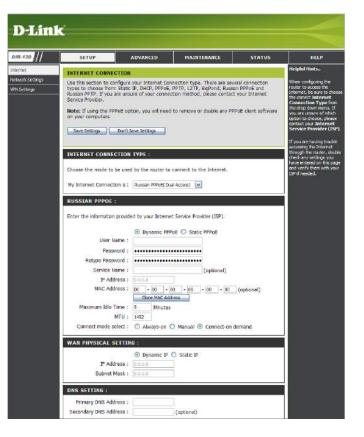
WAN Physical In most cases, select Dynamic PPPoE. Select Static PPPoE if your ISP assigned you the IP address, subnet mask, gateway, Setting: and DNS server addresses.
