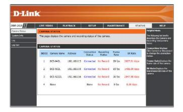
**Note:** If the Frame Rate or Bit Rate is too low, check the your network configuration between cameras and NVR. If the bit rate is too high, it will cause the Live Video display to slow down or lag. You should modify the quality or bit rate setting in the camera web GUI accordingly.
