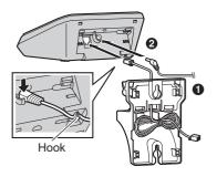
3 Insert the hooks on the wall mounting adaptor into the holes ♠ and ♠ on the base unit.
