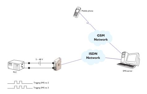
Configure a IDW-90 to send different SMS depending on the I/O input pulse train.
