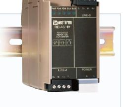
The RD-48 is a multi-purpose device that allows the extension of networks beyond the normal scope of the RS-422/485 standards. The device can be used as a repeater to extend the maximum distance of a network beyond 1200 m or the number of devices above 32. It can also swap between 2 and 4 wires or be used to build a structured and isolated net-
