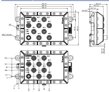
Weight 0.9 kg Degree of protection IP65
